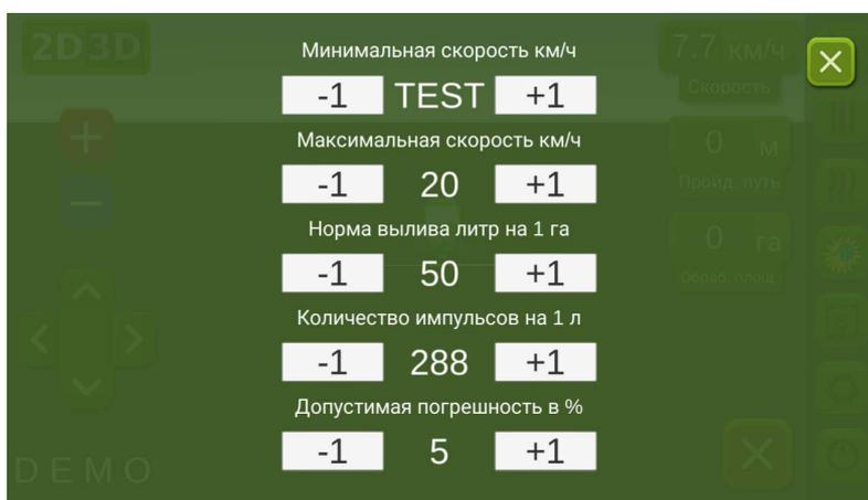
the metering valve will change inversely, from maximum to minimum (at high speeds).
